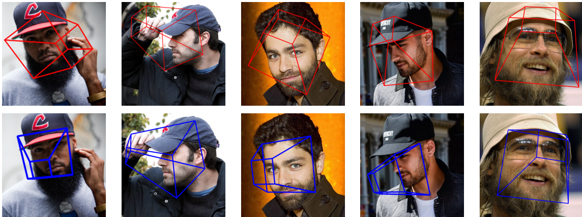
Figure 5.8: Estimation of head pose using three different models (all trained on BIWI), on unseen images taken from the web. Top row: Results for CNN-based model [10] which takes RGB images as input, Bottom row: Results for GCN-based framework which takes locations of keypoints as input. It can be seen that our GCN-based model generalizes much better than a CNN-based model directly trained on face images.
